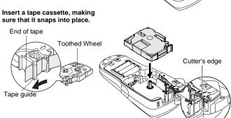
Make sure that the end of the tape feeds under the tape guides. • If the ink ribbon is loose, use your finger to wind the toothed wheel in the direction of the arrow on the cassette.
